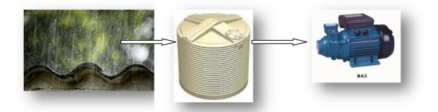
Rain falls on the roof and gets piped to a water tank (Like sun on solar panels). The more roof area, the more rain gets collected. The water tank stores rain water, like a battery stores electricity. We need to only use the water tank at about 10% a day in case we have periods without rain. On the output the tank a pump pushes out water, like an inverter pumps out power. The size of the pump is dependent on the number of taps that are on at one time.
